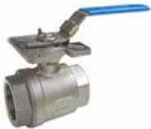
VBM2D 2PC Ball Valve 1000WOG, Full Port, ISO 5211 Direct Mount Size: 1/4" - 2"
